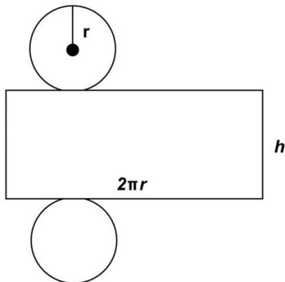
This is made up of its curved surface area plus its two circular ends
