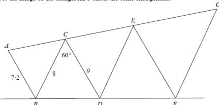
The proposed dimensions for the structure are |AB| = 7.2 m, |BC| = 8 m, |CD| = 9 m and  $|\angle DCB| = 60^{\circ}$ .
