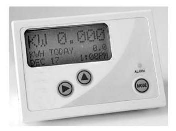
The kilowatt-hour is the unit of electrical energy used by electricity suppliers. The photograph shows a kWh (kilowatt-hour) meter. This meter is connected into the electricity consumer's domestic circuit and it can measure energy consumption in a selected part of the circuit, the total energy used and cost it. The meter can be wall-mounted in a convenient place.
